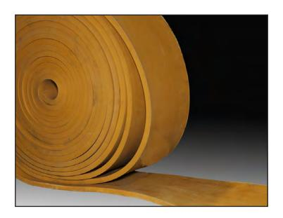
Many companies use industrial skirting rubber that has a hardness of 65-70 durometer, which can cause top cover belt damage. PangSkirt 45 is produced using a 45 durometer natural rubber blend. This will result in less belt wear and longer belt life.
