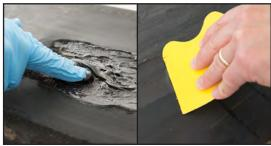
Work a thin layer of Eli-Flex into the prepared surface with your fingers. Continue spreading Eli-Flex using a spatula or any other flat-edged tool. Working time is approximately 20-30 minutes. After approximately 45 minutes the resin will gel, and after 120 minutes it will set. It is now ready for belt operation, but will take 8-10 hrs to reach full strength.
