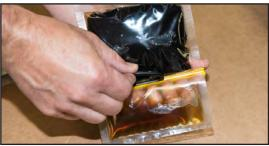
Remove the resin pouch and lay flat. Grasping the pouch on either end, gently pull the two sides apart until the separator tube pops up. Pull the tube out, moving from top to bottom.
