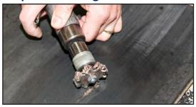
Prepare the damaged conveyor belt surface by removing loose rubber and grinding the surface. We recommend the Rubber Terminator drill mounted disk. Ensure the surface is cleaned, roughened and free of dust, oil, grease and moisture. Only use solvent before roughing process to clean contaminated surface.
