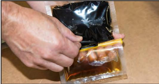
Remove the resin pouch and lay flat. Grasping the pouch on either end, gently pull the two sides apart until the separator tube pops up. Pull the tube out, moving from top to bottom.
