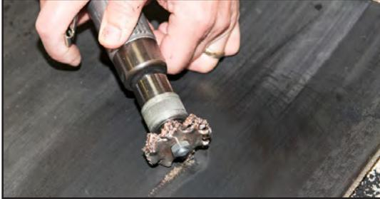
Prepare the damaged conveyor belt surface by removing loose rubber and grinding the surface. We recommend the Rubber Terminator drill mounted disk. Ensure the surface is cleaned, roughened and free of dust, oil, grease and moisture. Only use solvent before roughing process to clean contaminated surface.
