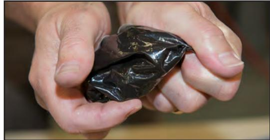
Mix the hardener and resin together for approximately 2-4 minutes by working the bag in your hands. The resin will start to warm up after 2-3 minutes of mixing. In winter, mix for 4-5 minutes.
