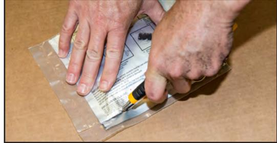
Feel the aluminum foil for the clip separator inside. Cut the foil along the edge to the outside of the separator clip.
